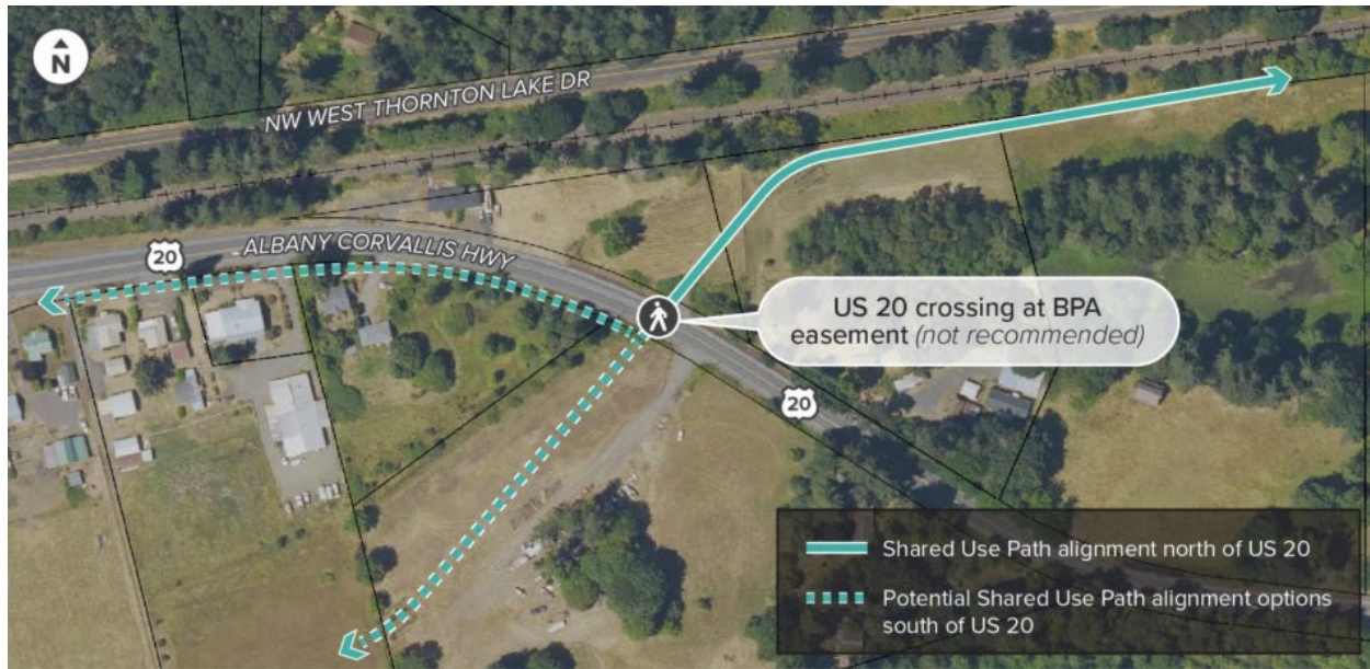
Figure 36. BPA Easement At-Grade Crossing Alternative
